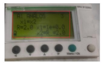
9) Then press right move button for changing A1 value(A1=Low set point of 1<sup>st</sup> pump), as shown in below image:-
