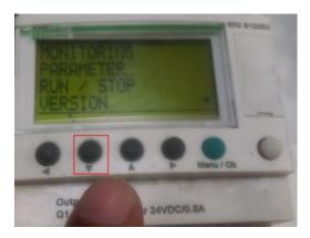
6) After that Parameter text will be selected and it will be in the blinking state as shown in below image:-
