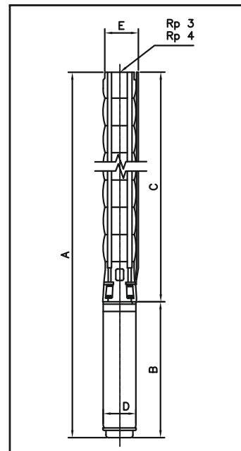
QF 75 - 20 to QF 75 - 24 are mounted in sleeve for Rp 3 connection.
