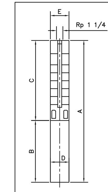
QF 5 - 56 to QF 5 - 75 are mounted in sleeve for Rp 1 1/4 connection
