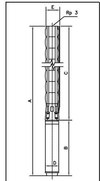
QF 50-24 to QF 50-39 are mounted in sleeve for Rp 3 connection.
