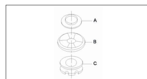
The stop ring, which is designed as a thrust bearing limits axial movements of the pump shaft.
